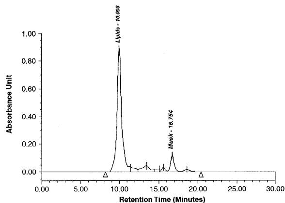
Fig. 2. Gel permeation chromatography showing residual lipids after alumina semi-clean-up of 2.09 g fish sample using PLE.
