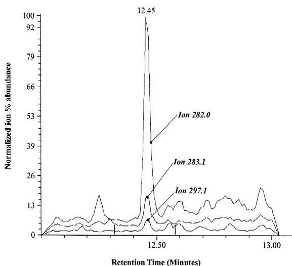
Fig. 3. Positive identification of musk xylene using ion chromatograms at  $m/z$  282.0, 283.1, 297.1, and retention time.
