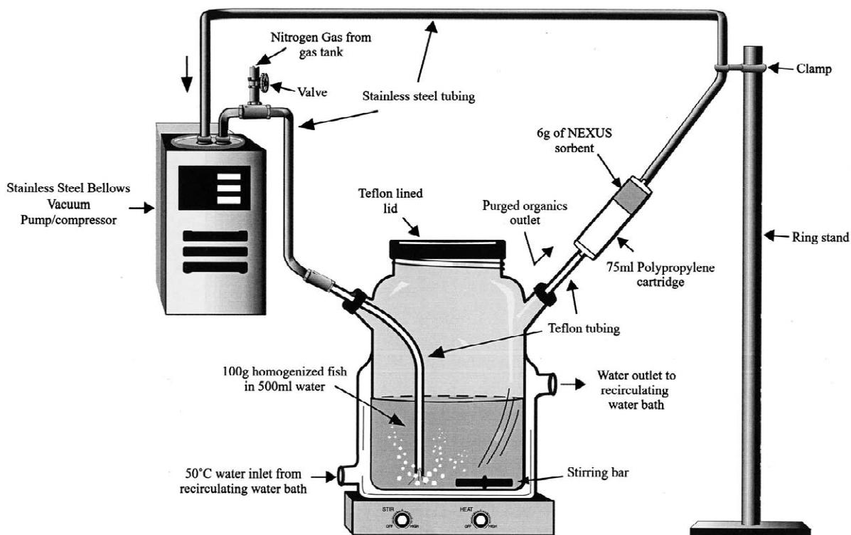
Fig. 1. Closed-loop stripping analysis apparatus.
